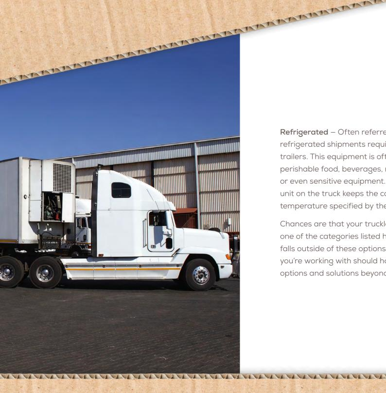
Refrigerated – Often referred to as "reefers," refrigerated shipments require temperature-controlled trailers. This equipment is often used to haul perishable food, beverages, medicine, plants, or even sensitive equipment. The refrigeration unit on the truck keeps the cargo at the exact temperature specified by the customer.
